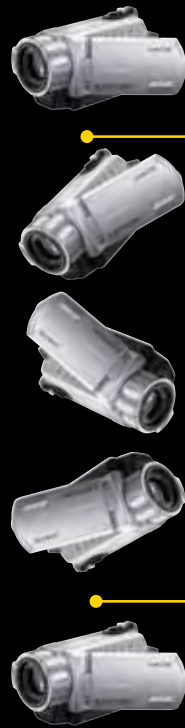
3G Sensor detects fall. Write-head retracts.
