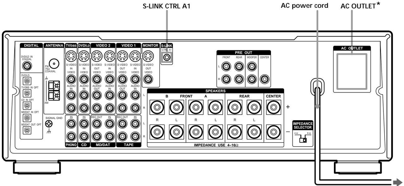
\* The configuration, shape, and number of AC outlets on the rear panel varies according to the model and country to which the receiver is shipped.
