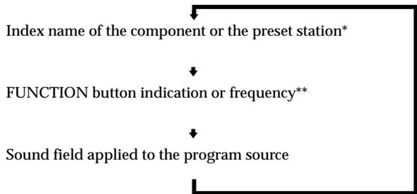
\* Index name appears only when you have assigned one to the component or preset station (see page 42). Index name does not appear when only blank spaces have been entered, or it is the same as the function button.
