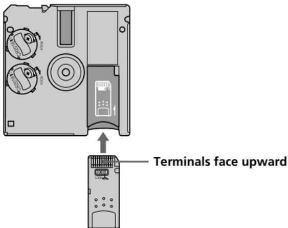
Make sure that “Memory Stick” is seated securely in the floppy disk adaptor. Otherwise, it will not work correctly.
