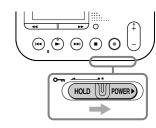
Slide the HOLD-POWER switch in the direction of "POWER" and keep it there until "关机" animation appears.
